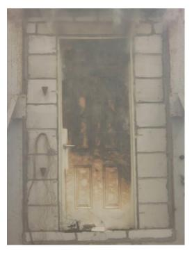
Fig. 5 Unexposed Side after 20 Minutes
