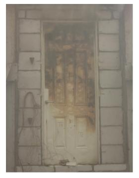
Fig. 4 Unexposed Side after 16 Minutes
