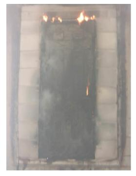
Fig. 6 Exposed Side after 20 Minutes
