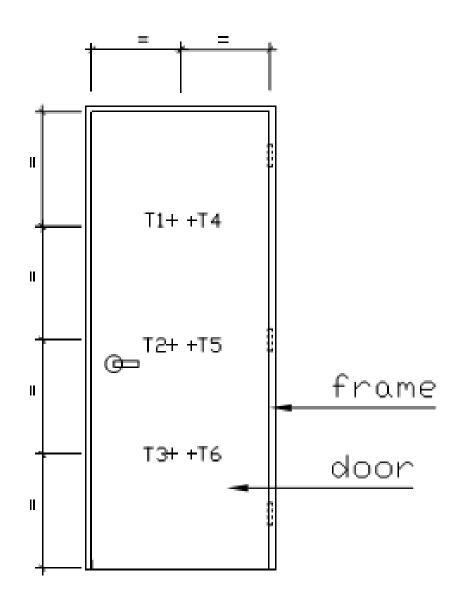
POSITON FOR MEASUREMENT OF UNEXPOSED TEMPERATURE
