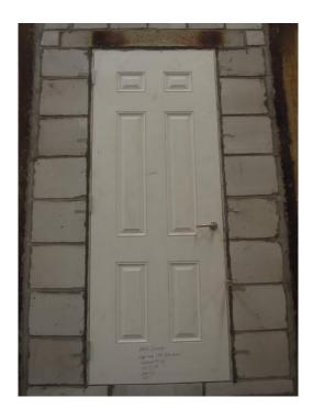
Fig. 1 Exposed Side Prior to the Fire Test
