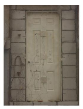
Fig. 3 Unexposed Side after 10 Minutes
