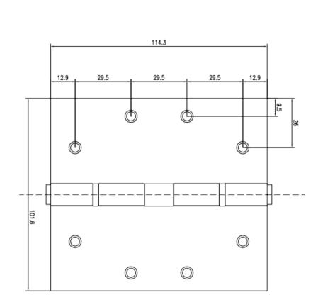
Irem No: 55039A Material: SUS304 Finish: SS Dimension(H×W×T):4.5"×4"×3.4mm
