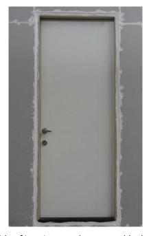
Fig. 2 Unexposed Side of inswing test door assembly during air leakage test
