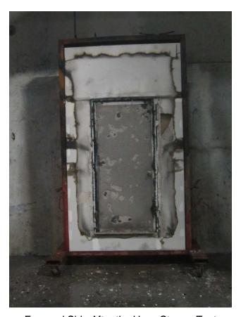
Exposed Side After the Hose Stream Test
