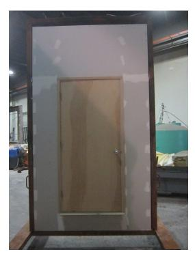
Exposed Side Prior to the Fire Test
