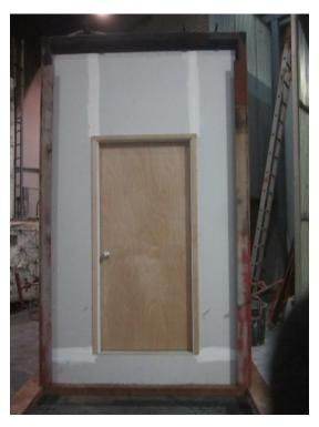
Unexposed Side Prior to the Fire Test
